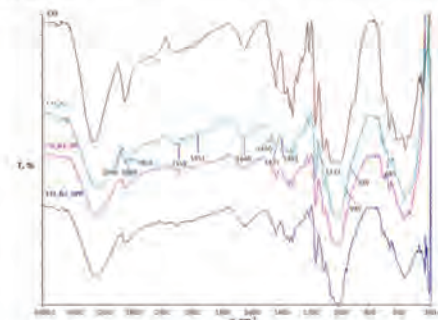
Figure 1. FTIR spectral bands of chitosan finished cotton fabric before and after maintenance cycles compared to untreated fabric
